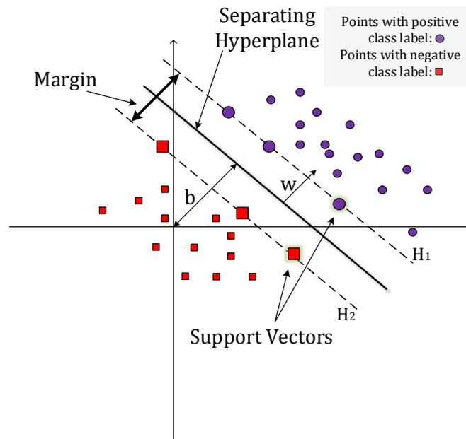
**Figure 2.** Optimal separating hyper plane.
